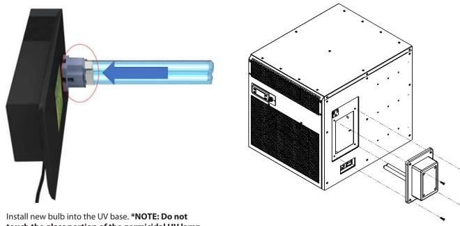
Install new bulb into the UV base. \*NOTE: Do not touch the glass portion of the germicidal UV lamp with bare hands. Use cotton gloves or rag to avoid skin oils that will harm the UV lamp.
