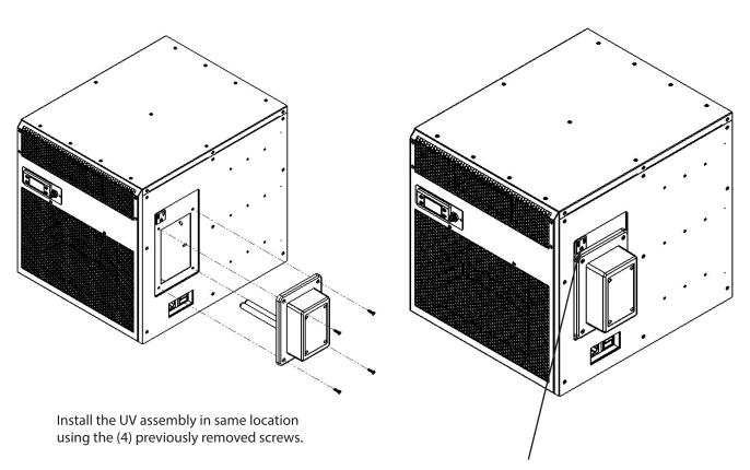
Plug the UV assembly power cord into the UV power receptacle
