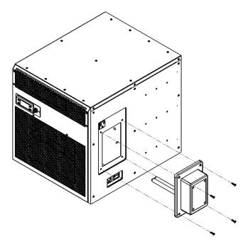
Remove the (4) screws and UV assembly.
