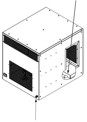
\*Do not insert drain line brush in the exterior drain port.
