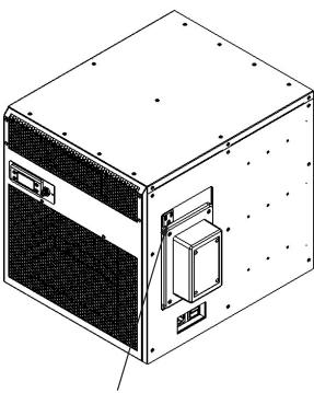
Unplug the UV assembly power cord from the UV power receptacle
