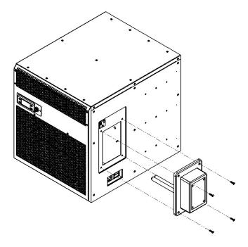
Remove the (4) screws and UV assembly.
