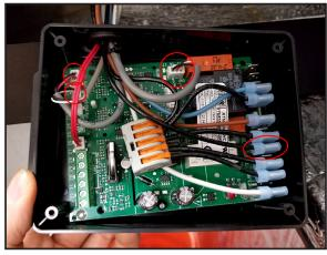
Disconnect Pb1, Pb2, Display, and flag connector from terminal #6. Next, remove the wires from the enclosure as shown.
