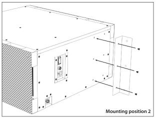
**STEP 5**Foam tape needs to be placed on bracket surfaces which will be in direct contact with the wall.
