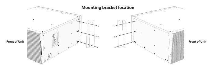
**STEP 4**Secure the two brackets to the corresponding side of the cooling unit on exterior side of the cellar. There are two mounting positions available.
