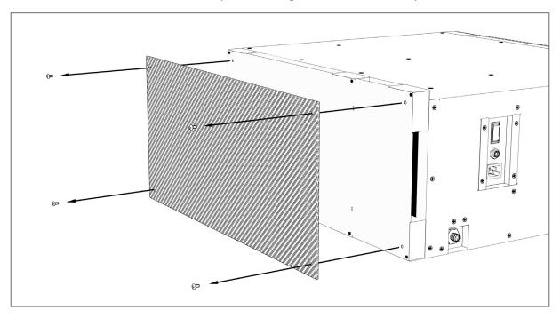
**STEP 2**Remove the 6 screws securing the grille to the unit. The grille can now be removed from the unit.
