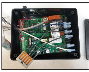
Disconnect Pb2, DI, Display, and Pb1 wires from the circuit board.
